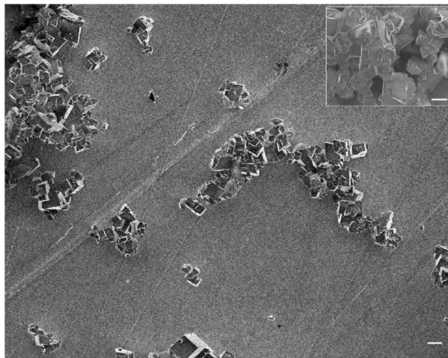
Fig. 3 SEM image of neat calcium carbonate nanoparticles demonstrating a rhombohedral crystalline structure and nanoparticle aggregation. Inset image confirms the presence of non-uniform \text{CaCO}_3 particles. Scale bars on the main and inset images represent 10 microns.
